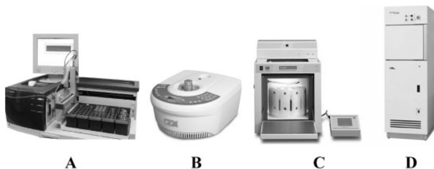
Figure 1. Microwave reactors for chemical syntheses. A: Emrys Liberator (Biotage, Sweden, www.biotage.com ); B: CEM Discover BenchMate (CEM, USA, www.cem.com ) Copyright CEM Corporation; C: Milestone Ethos TouchControl (Milestone, Italy, www.milestonesci.com ); D: Lambda MicroCure2100 BatchSystem (Lambda, USA, www.microcure.com ).
