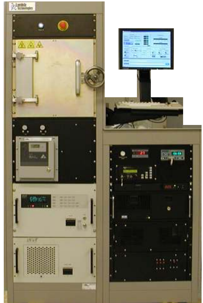
MC3100 configured with 2KW HPA for higher power applications
