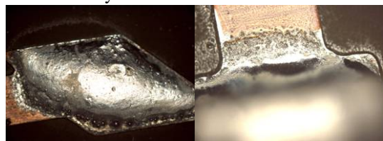
Figure 9. SnPb formed at 230 °C by VFM
