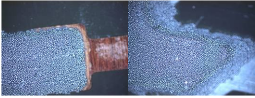
Figure 6. SnAg alloys on Cu and Sn formed at 250 °C in the thermal reflow.
