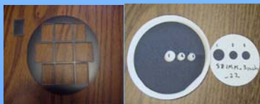
Left: Rectangular pieces and circular disks cut from the deposited diamond. The rectangular pieces are 12 x 18 mm. The diameter of the circular disc #1 is 0.5 inch or 12.7mm. The other two circular discs are 9mm in diameter.
