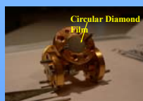
A 36 μm thick circular freestanding polycrystalline unpolished diamond film mounted on the microwave transmission test structure.
